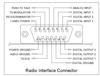
See section 4 for more complete details on proper interfacing to your repeater transmitter and receiver.
