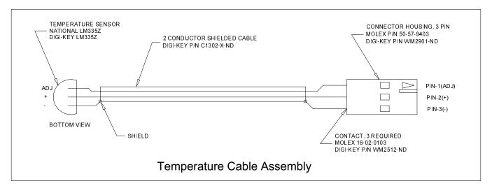
Plug the temperature sensor cable assembly into the connector labeled "Temp" on the RI-300 or RI-310. Next to the temperature connector is an adjustment that can be used to calibrate the temperature. You will need a reference temperature for this calibration. Do not mount the sensor to the TX heat sink for calibration.
