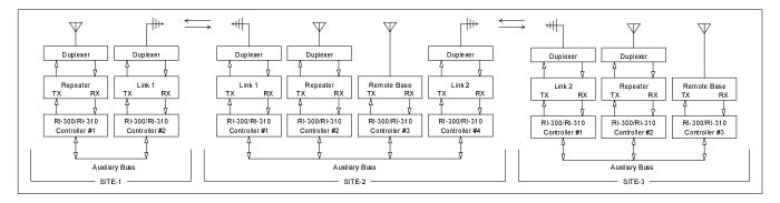
In systems like these, using the RI-300/RI-310 controller makes it possible to both use telephones and control remote base radios between sites. Site 1 could even use a remote base radio on site 3 without interfering with the repeater operation of site 2. The RI-300 is so flexible that you can add or move links from any site without impact to the rest of the system.
