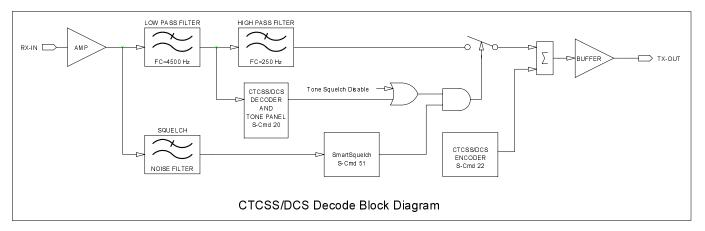
The above block diagram shows how the repeat audio is processed through the controller. This command sets up the Tone Panel shown in the diagram. Notice that the Tone Squelch Disable, controlled by S-Command 01, is located after the tone panel.
