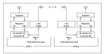
In our next example, we have added the ability to control the frequency and tone squelch of the link radio by adding a dedicated second controller to support these features. In this example, the link radio is better identified as a remote base radio. Users at each repeater can set the frequency of the remote base radio to allow a site to communicate with various other sites or even other repeaters, based on the frequency and the CTCSS tone used.
