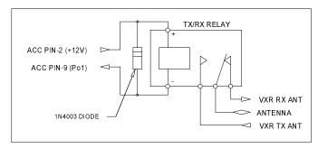
Two or more RI-310 controllers can be connected together via the auxiliary connectors. You can also connect two RI-310 controllers together via this 25-pin "ACC" connector, for linking or remote base operation. Use the following connections.
