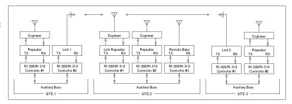
In our last example, we will use full duplex links between all sites. Each of these sites can include a repeater, remote base radio and telephone. In this example, users can talk to each other and pass control functions from site to site. The traffic on this type of link can be considered similar to a telephone party line. In this application, each repeater at each site can be connected or disconnected from the links.
